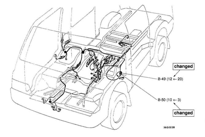
B-49 Front wiring harness and fuel gauge wiring harness combination
