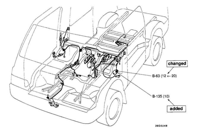
B-63 Front wiring harness and fuel gauge wiring harness combination B-135 Front wiring harness and fuel gauge wiring harness combination +
