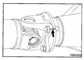
(2) With the mating marks in alignment, install the propeller shaft to the companion flange.
