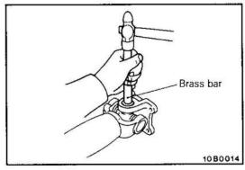
(2) Press the bearing and journal into one side with the brass bar.
