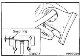
(3) Measure the clearance shown in the illustration with a feeler gauge. If the clearance exceeds the standard value, the snap rings should be replaced.
